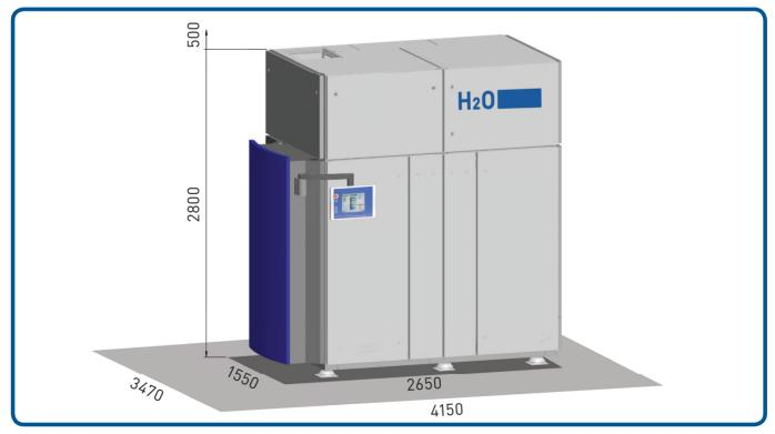
${\tt Dimensions\ of\ the\ VACUDEST\ vacuum\ distillation\ systems\ with\ optimal\ maintenance\ space}$
